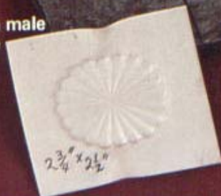
The shell or rosette design is pressed into the eight pieces of 20 gauge silver.
