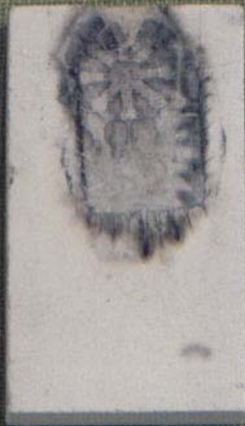
This piece of fire-clay composition soldering block was used as the flat half of the mold for all the castings on this page. It shows no apparent damage.
