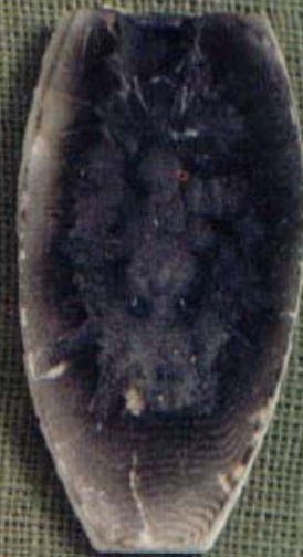
A design of a watch fob was carved into this cuttlebone and the metal poured without the surface of the mold having been coated. The hot metal almost destroyed the mold. A deep ripple design was left on the silver surface.
