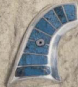
A lost wax centrifugally cast grip inlaid with turquoise
