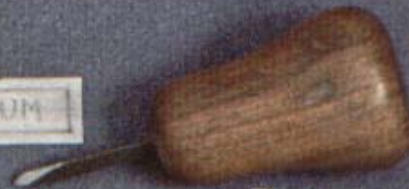
These two are homemade handles probably mesquite wood, with triangle file tips
