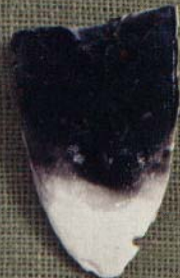
This brass model of a button was pressed into the cuttlebone. The mold was coated with a borax and water glass solution. When dry, it was coated with carbon from a torch. No burning away of the mold was noted until several buttons were cast. Before each casting the mold was thoroughly smoked.
