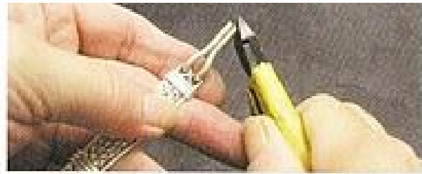
Figure 73 Cut sharp corners off to rough out an oval-shaped end.
