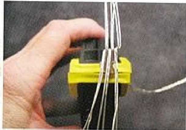
Figure 13 Wires back in place with about 1" woven.
