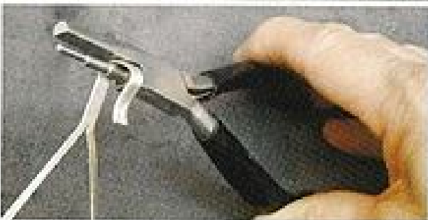
Figure 22 Shaping the bail.
