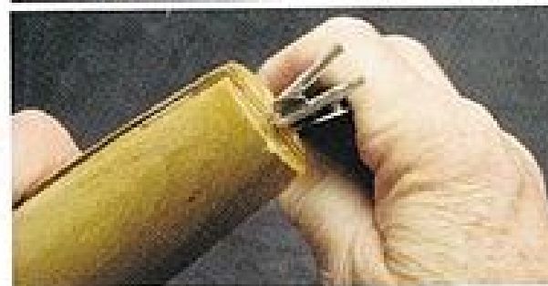
Figure 59 Use a penknife to separate the sawed wires.
