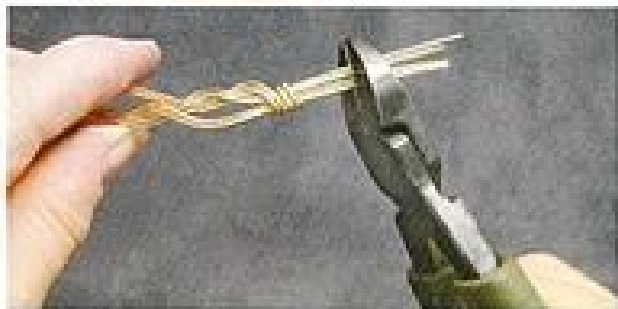
Figure 53 Cutting the wires.
