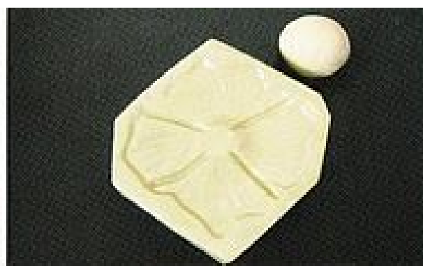
Figure 16 Pinch off a piece of PMC big enough to fit inside the mold.
