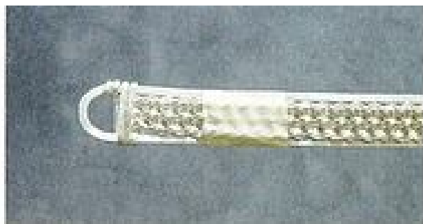
Figure 29 Back side after cutting wire, filing, and pressing the wire into place.
