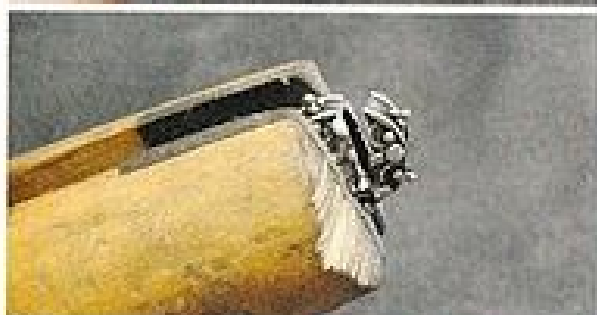
Figure 2 Saw off part of the bead.
