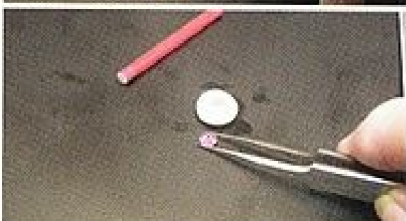
Figure 7 The center clay is removed. Ready to place the stone.
