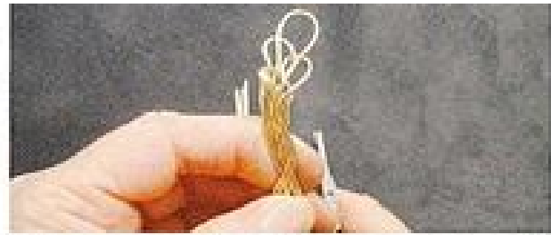
Figure 48 Wires tucked in. One remaining loop.
