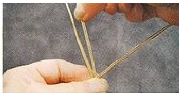
Figure 16 Grasp the intersection of the wires firmly.
