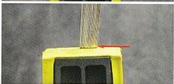
Figure 8 Move clamp to the \frac{1}{4} " (6 mm) mark.
