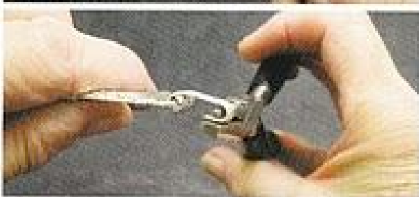
Figure 77 The pliers are now on the second step, as the curve needs to be wider.
