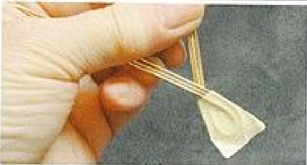
Figure 2 Wrap the loop with masking tape.
