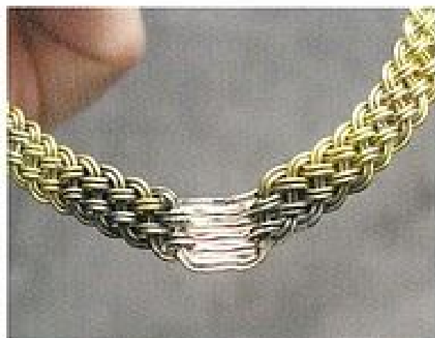
Figure 27 Back side— loose wires in the middle soldered.
