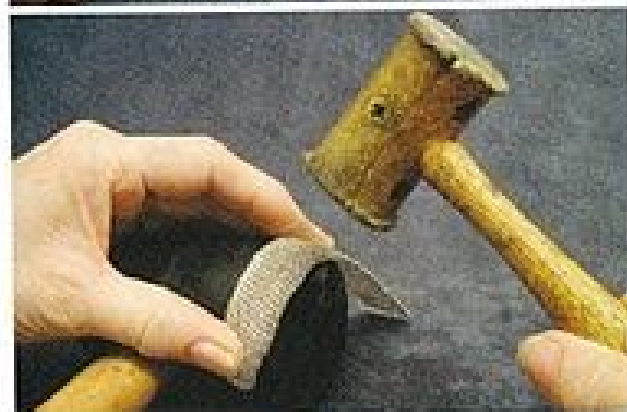
Figure 7 Beginning to dome the bracelet.
