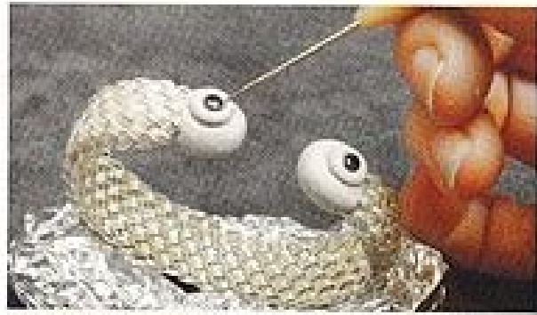
Figure 11 Clean and bevel the stone mounting.
