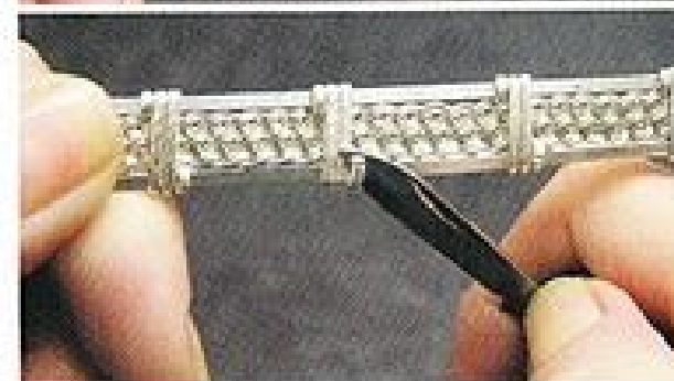
Figure 44 Back side of bracelet. Lift the end of the wire with a penknife.
