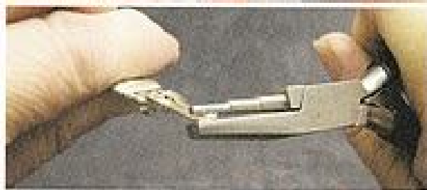
Figure 75 Make a slight upward curve at the very end of the clasp.
