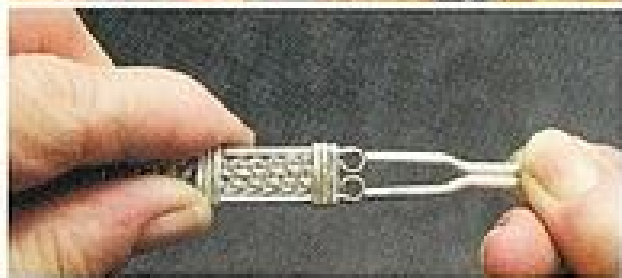
Figure 64 Both legs straightened. Check for fit with the loops at the end of the bracelet.
