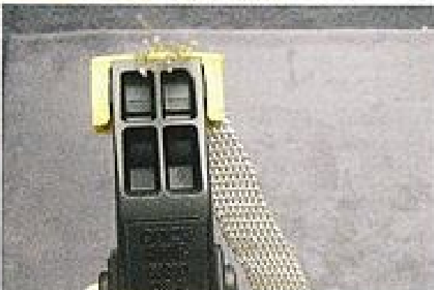
Figure 4 Almost through weaving. Wires must be kept straight.
