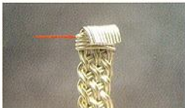
Figure 23 Back side. Flux and solder pieces go inside the bend, where the arrow is pointing.
